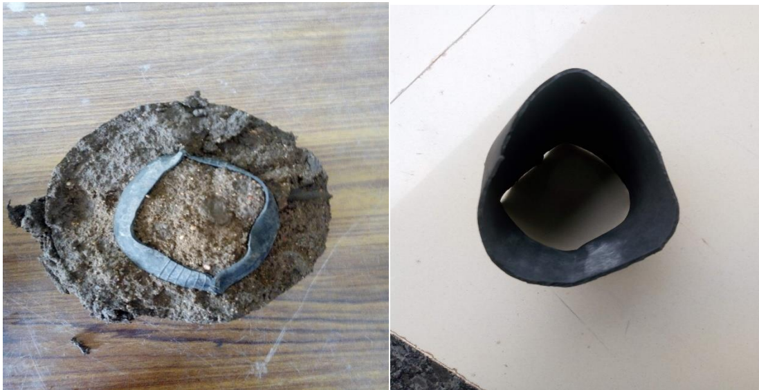
Fig 4 Geocell at 1/3H in Chevron pattern
