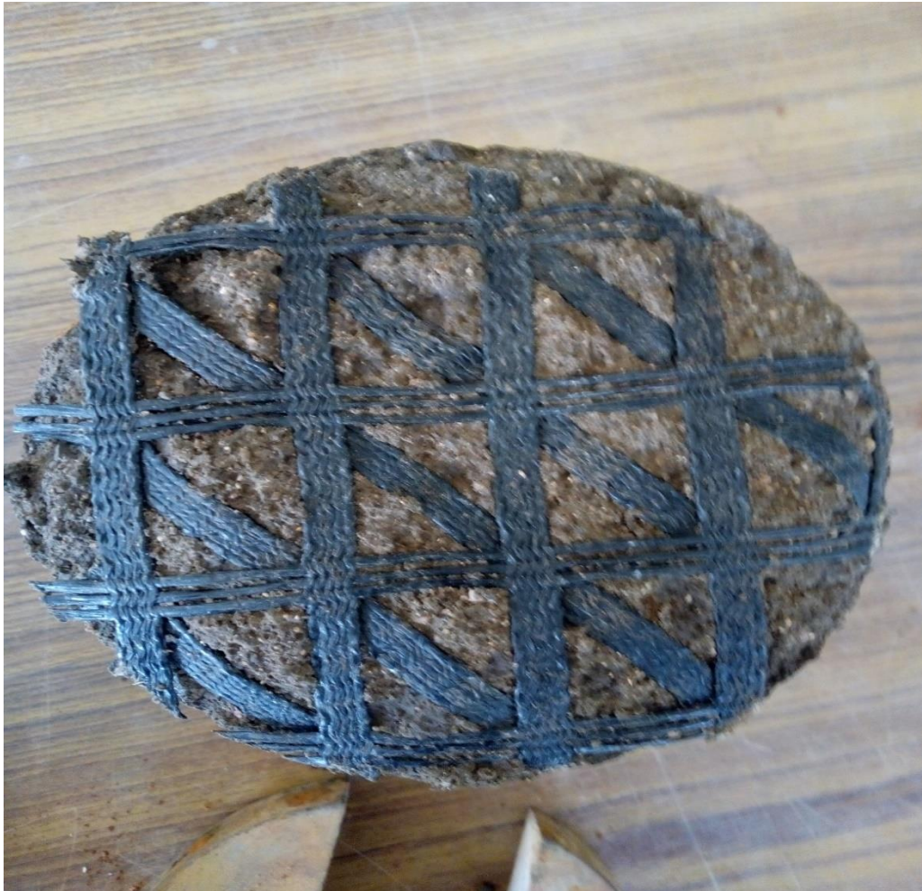
Fig 10 Triaxial geogrid at 1/3H after CBR test
